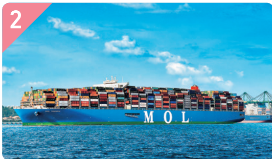
20,000 TEU-class containership. LOA: 400m, breadth: 58.8m ※ Current ship name and hull are different from the above image.
