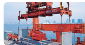
Flat rack container Transporting long, heavy-weight, or oversized cargo, which cannot be accommodated in a standard container
