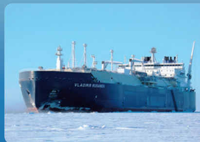
Icebreaking LNG carrier. Tank capacity is 172,000m 3
