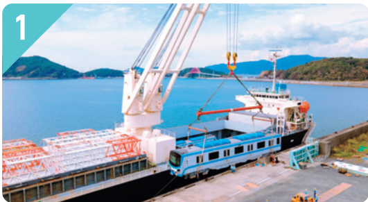
A heavy lifter loading subway cars
