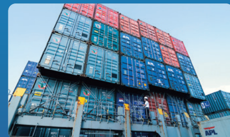
Crewmembers on a lashing bridge check loaded containers
