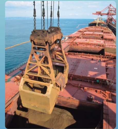
Iron ore carrier discharging cargo
