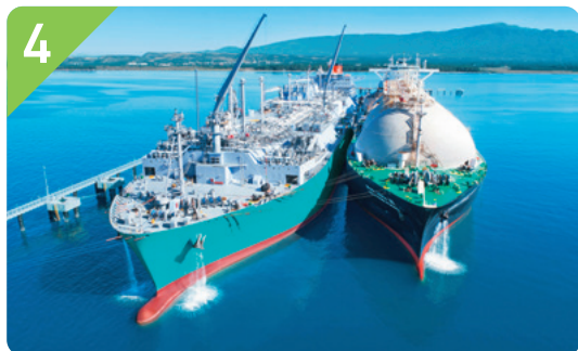
Floating storage & regasification unit (FSRU)
