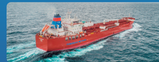
A methanol and heavy oil dual-fuel methanol tanker, emblazoned with "Powered by Methanol" on the hull
