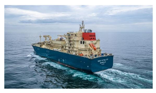
The 18,600-m³ newbuild bunker vessel is TotalEnergies Marine Fuels' second collaboration with shipowner Mitsui O.S.K. Lines, Ltd (MOL) and shipbuilder, Hudong-Zhonghua Shipbuilding following the signing of a long-term charter contract in November 2019. All three parties first collaborated in 2018 to successfully design and build her sistership, the Gas Agility, which has been operating in the Port of Rotterdam since November 2020.
