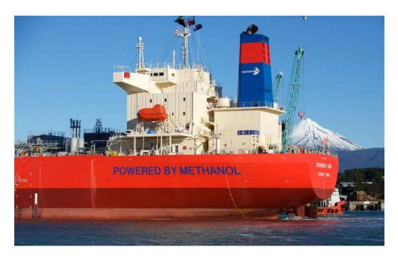
"Taranaki Sun" Methanol Dual-fueled Methanol Carrier Vessel
