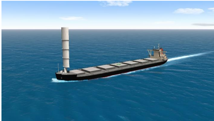
CG simulation of coal carrier underway with Wind Challenger
